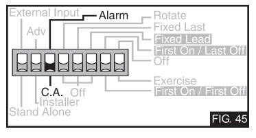
The Rotate / Off DIP switch selects whether or not the control is to provide Equal Run Time Rotation of the boiler stages. If the switch is set to Rotate, the stages will be rotated accordingly. If the switch is set to Off, the firing sequence is fixed starting with the lowest stage to the highest stage (FIG. 46).
